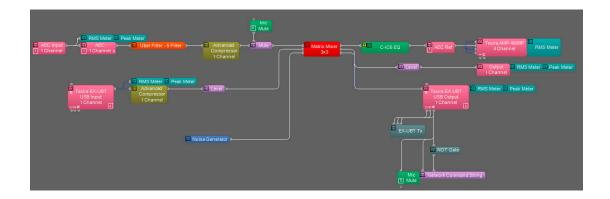
The EX-UBT is configured for Speakerphone: Disables Computer AEC. In this mode Teams will offload its AEC processing and allow Tesira to handle this exclusively.
