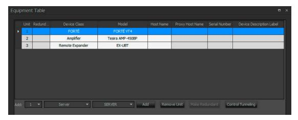
In the file, the matrix routing is already in place to support the room design requirements. A single AEC input channel on the TesiraFORTÉ AVB VT4 will support the connection to the TeamConnect Ceiling 2 via the Dante to analog convertor. A single analog output channel will be used to route a reference signal back to the TeamConnect Ceiling 2 via the analog to Dante converter.
