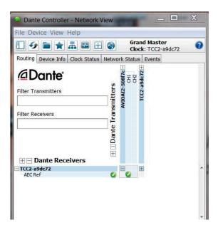
In order to improve the AEC-performance of the overall conference setup it is advisable to provide the AEC-reference signal (i.e. as being played back by the loudspeakers) to the TeamConnect Ceiling 2's reference-input-channel (1st Dante input-channel), so the beam-steering can be stabilized during far end speech.
